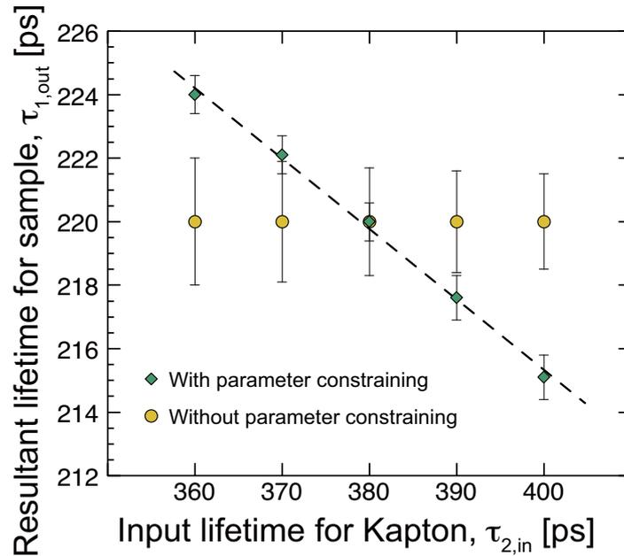
**Fig. 1.** Variation of  $\tau_{1,out}$  analyzed with and without constraining the 2nd lifetime as a function of  $\tau_{2,in}$ . The broken line represents the result of a linear fit for the data with parameter constraining. The error bars denote the twice width of the respective standard errors from the LSF analysis.
