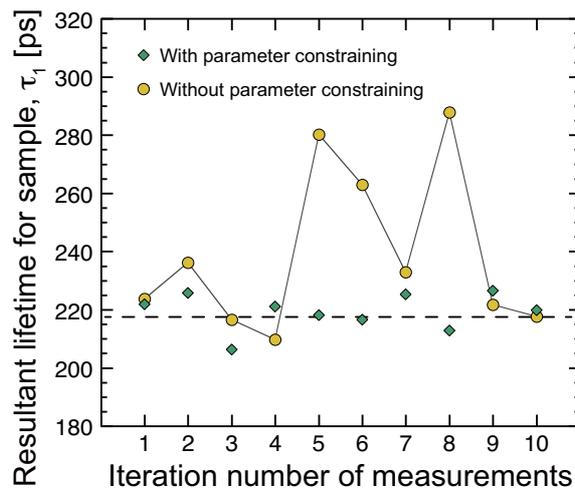
**Fig. 3.** Variation of  $\tau_1$  for the data of 20 k counts, analyzed with and without constraining the 2nd lifetime, as a function of measurement number. The broken line represents the average value of 219 ps for  $\tau_1$  analyzed with parameter constraining. The solid line is drawn to guide the eye.
