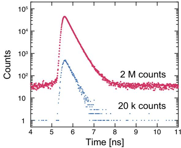
**Fig. 2.** PAL data for the single-crystal silicon, experimentally measured with different accumulation statistics (red dots: 2 M counts, blue dots: 20 k counts).
