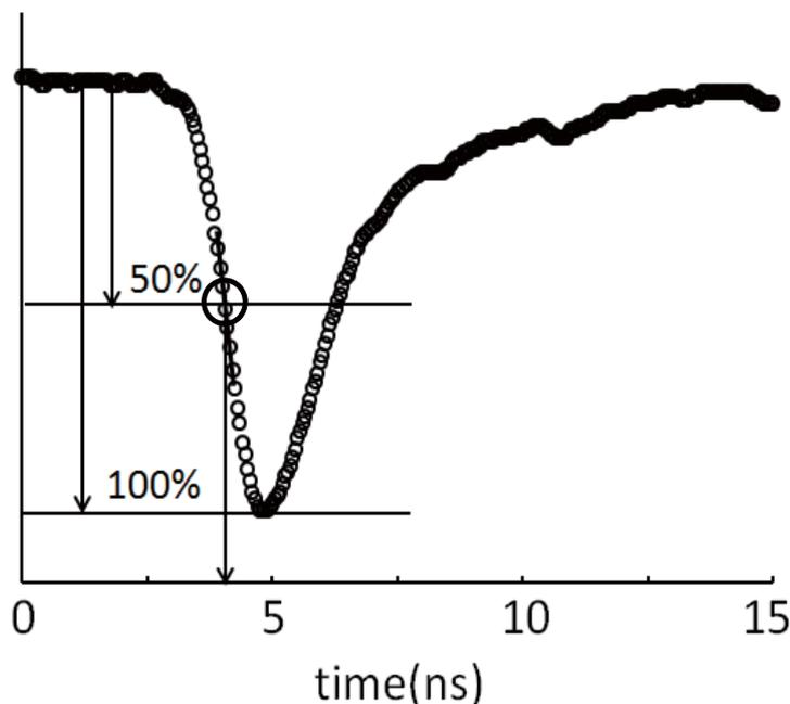
**Fig. 1.** Wave form from one of the scintillation detectors measured by a DSO. The time information of this signal was obtained at the crossing point indicated by the circle.
