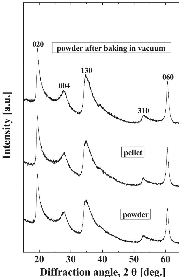
**Fig. 1.** XRD patterns observed for conventional powder (bottom), pellet prepared by uniaxial compaction (middle), and powder after baking at 423 K for 12 h in vacuum of  $10^{-3}$  Pa (top).
