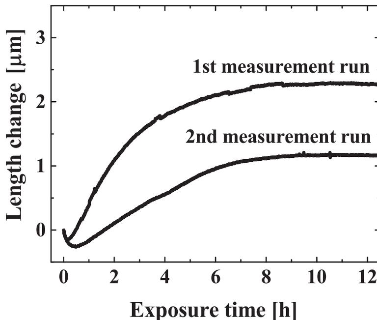
**Fig. 2.** Length changes of saponite layered nanoparticles as a function of exposure time obtained in the 1st and 2nd measurement runs. See text as for the description of the measurement run conditions.
