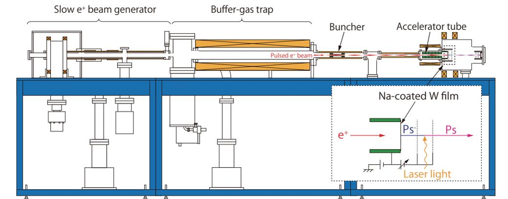
**Fig. 8.** Conceptual design of the positronium beam utilizing the trap-based positron beam.
