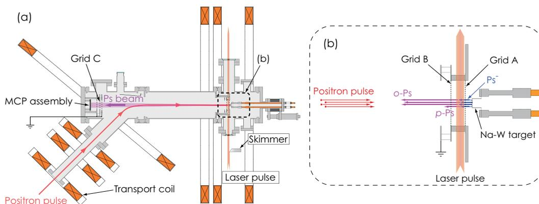
**Fig. 1.** (a) Apparatus for the positronium beam production, (b) schematic view of the photodetachment region (not to scale) [12].
