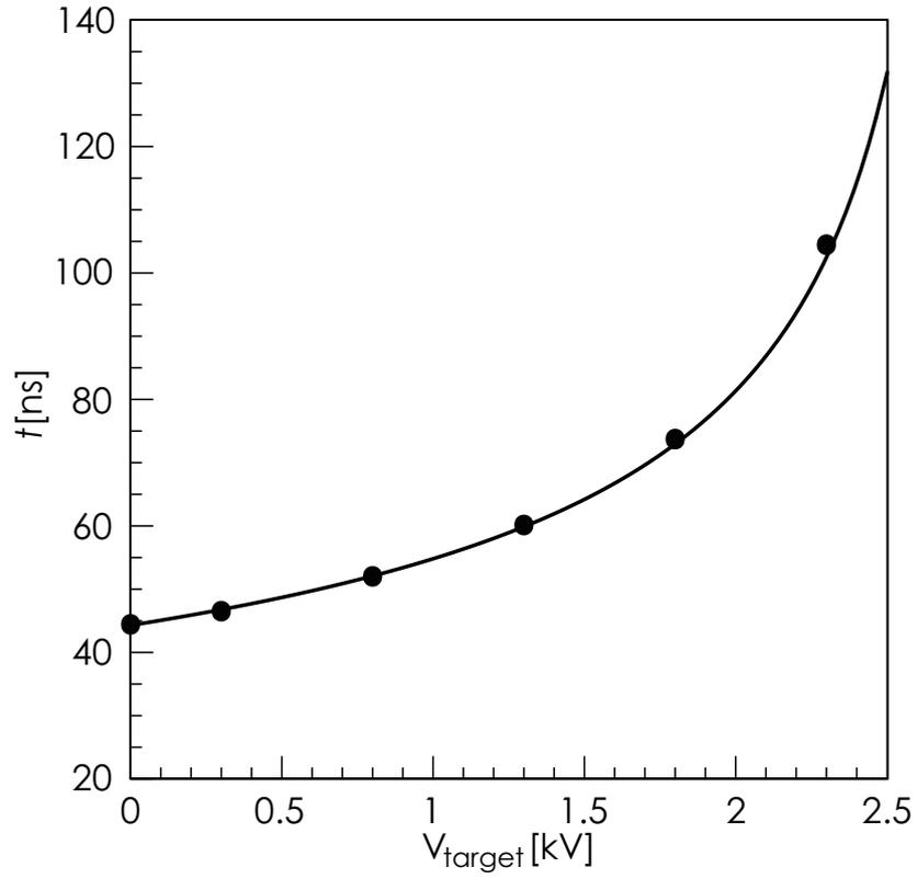
**Fig. 5.** TOF obtained from Fig. 4 as a function of the target bias,  $V_{\text{target}}$  [12]. Solid curve shows the TOF of the positronium calculated using Eq. (2).
