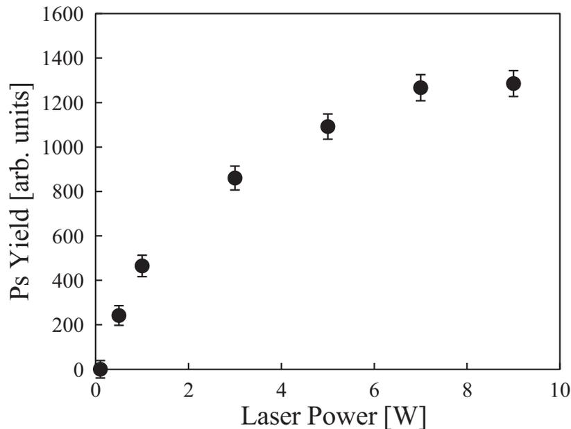
Fig. 7. Positronium yield as a function of the laser power, with  $V_{\text{target}} = 1.3$  kV.
