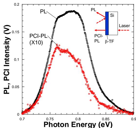
**Fig. 3.** PL and PCI-PL spectra for Cu-doped  $\beta$ -FeSi<sub>2</sub> thin film/Si (see the inset). The PCI-PL spectrum includes information of migration of minority carrier (hole) with a repeated trap process and radiative recombination efficiency of electrons and holes at the
