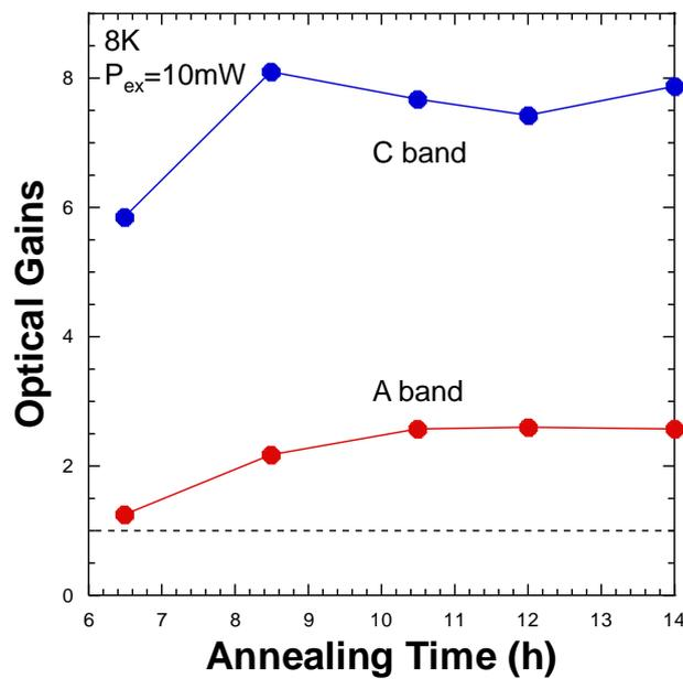
**Fig. 2.** Optical gains (ratio of intensity enhanced) for the A and C bands emissions as a function of annealing duration (time). Each peak intensities of the A and C bands were obtained by analysis of spectral peak separation.
