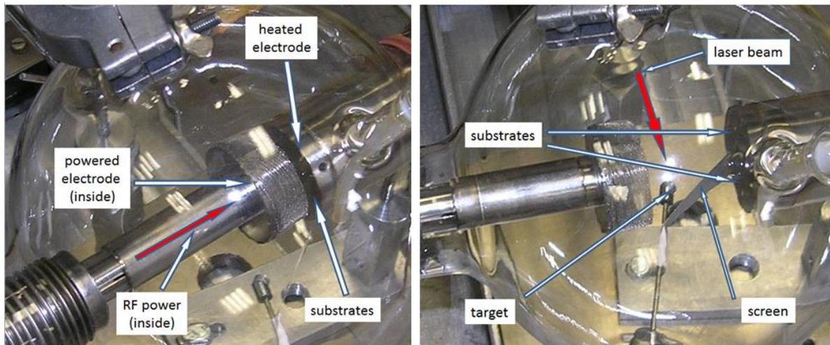
Fig. 1. Deposition chamber for *in situ* deposition at condition PECVD and RLA
