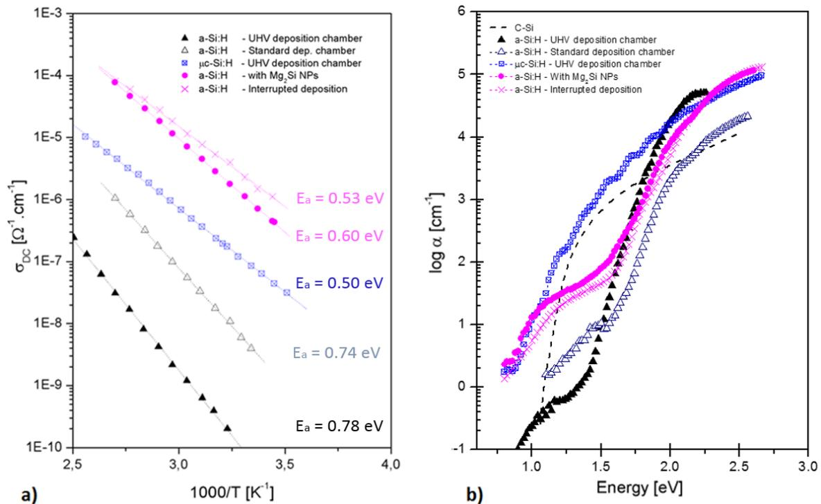
Fig. 3. Temperature dependences of electrical conductivity of the deposited thin films (a) and absorption coefficient as a function of energy of photons of a-Si:H thin films deposited at different conditions (b)
