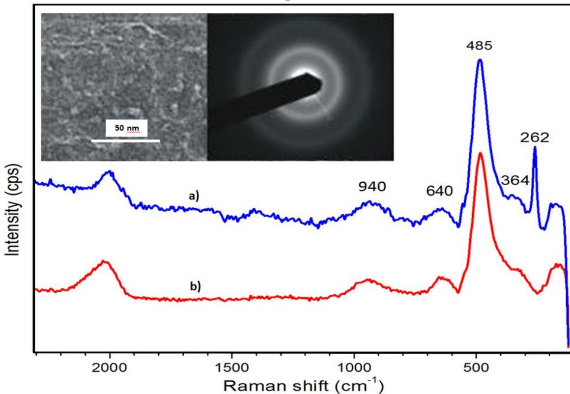
Fig. 2. Raman spectra of the deposited films, structure A, a-Si:H/Mg<sub>2</sub>Si/a-Si:H film (a) and structure B, only a-Si:H layer (b). Left inset: HRTEM image of the deposited structure A, Right inset: corresponding selected electron diffraction pattern.
