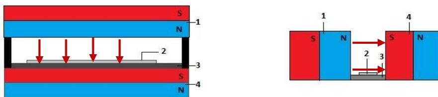
**Fig. 1** Sample drying in a magnetic field: 1,4 – ferrite magnets with a constant magnetic induction  $B = 0.2\text{--}0.3\text{ T}$ ; 2 – composite layer; 3 – substrate, arrows show direction of magnetic field
