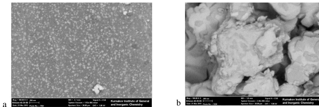
**Fig. 3** Micrographs of ferrite-cobalt shell (a) and modified  $\text{BaTiO}_3$  particle (b)
