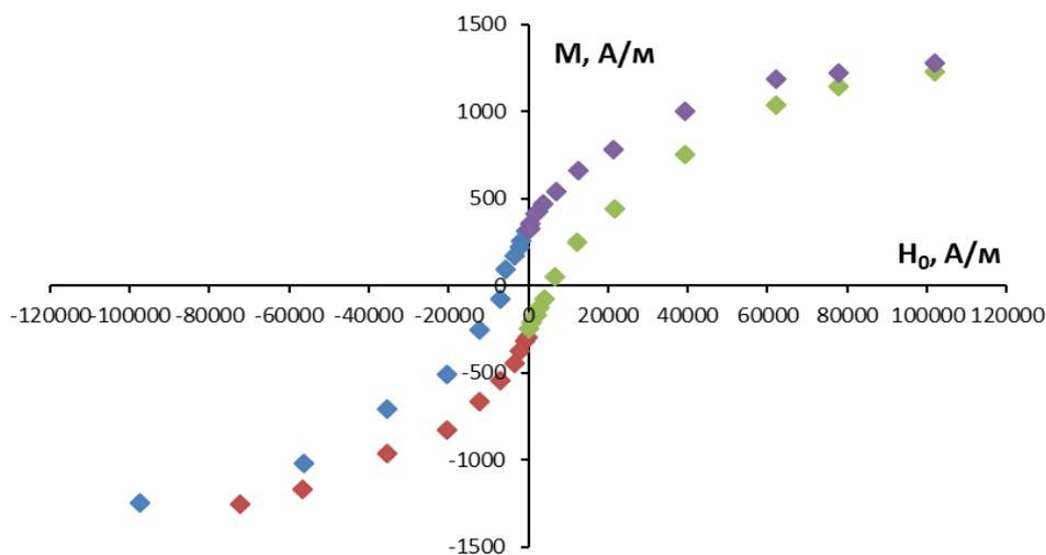
**Fig. 4.** Magnetization plot of  $\text{BaTiO}_3$  particles encapsulated with a  $\text{CoFe}_2\text{O}_4 - \text{SiO}_2$  shell
