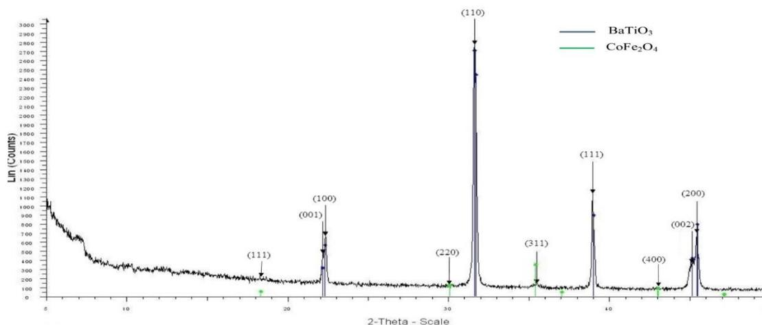
**Fig. 2** The XRD pattern of  $\text{BaTiO}_3/\text{CoFe}_2\text{O}_4\text{-SiO}_2$  particles
