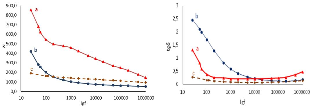
**Fig. 5** Frequency dependence of dielectric permittivity for CEPVA- $\text{BaTiO}_3$  core/shell (20,3 vol.% of  $\text{CoFe}_2\text{O}_4$ ) composites dried under the impact (a) and in the absence (b) of a magnetic field in comparison with the composite obtained using a non-modified commercial  $\text{BaTiO}_3$  filler (c)
