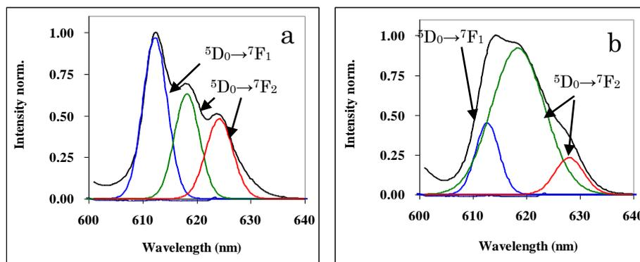
**Fig. 4.** Photoluminescence spectra of  $\text{ZnAl}_2\text{O}_4$  based phosphors prepared by solution-combustion (a) and sol-gel method (b) with 7 %  $\text{Eu}^{2+}$  concentration.
