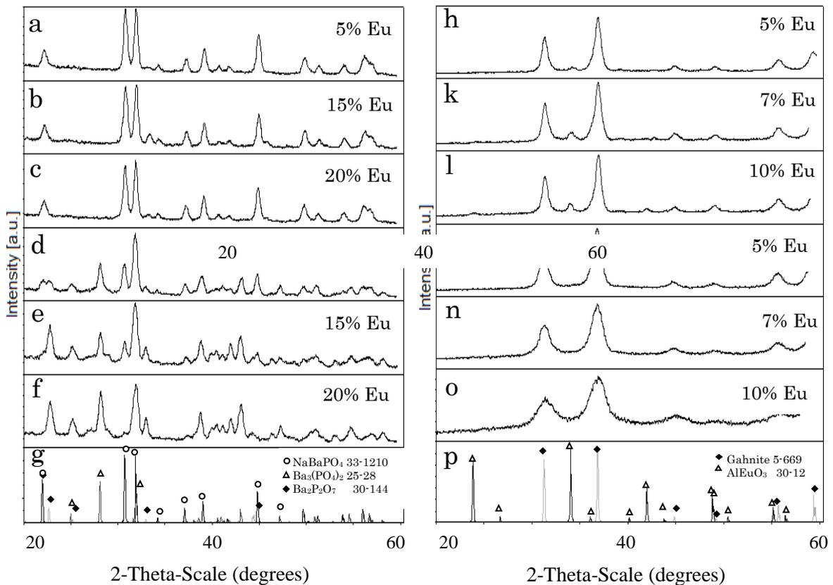
**Fig. 1.** XRD patterns of NaBaPO<sub>4</sub> phosphors prepared by SC (a,b,c) and SG method (d,e,f) and ZnAl<sub>2</sub>O<sub>4</sub> phosphors prepared by SC (h,k,l) and SG method (m,n,o); (g,p)-PDF data.
