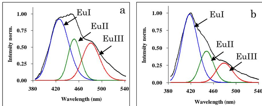
**Fig. 2.** Photoluminescence spectra of  $\text{NaBaPO}_4$  based phosphors prepared by solution-combustion (a) and sol-gel method (b) with 15 %  $\text{Eu}^{2+}$  concentration.
