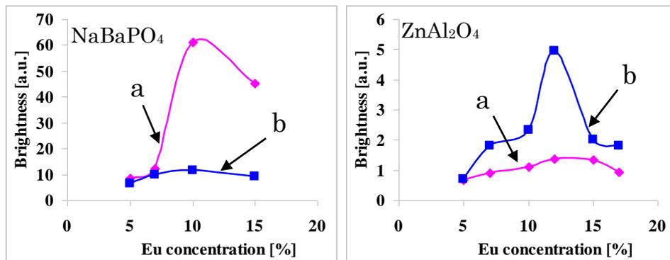
**Fig. 3.** Brightness depending on Eu content in  $\text{NaBaPO}_4$  and  $\text{ZnAl}_2\text{O}_4$  phosphors prepared by solution-combustion (a) and sol-gel method (b).
