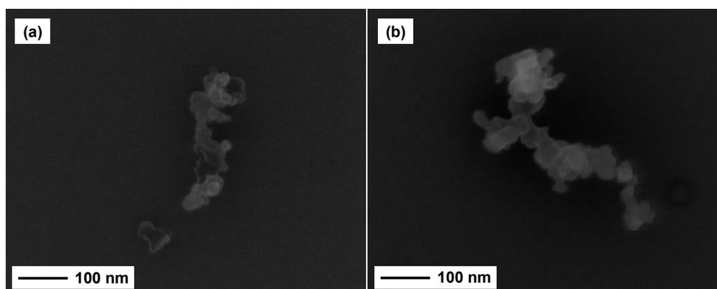
**Fig. 2.** Morphology of natural nanofillers prepared by the ammonium persulfate oxidation method: (a) bleached birch Kraft pulp and (b) birch bark.
