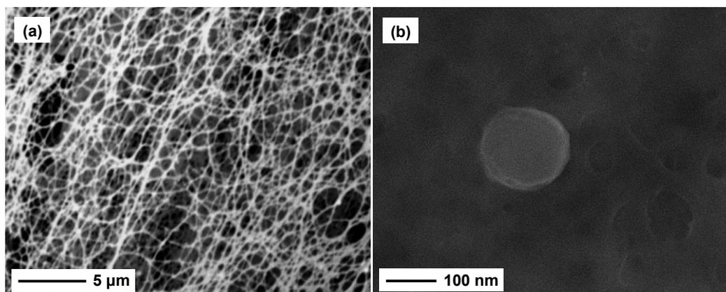
**Fig. 1.** Morphology of bacterial cellulose after: (a) alkaline treatment and freeze drying and (b) oxidation with ammonium persulfate.
