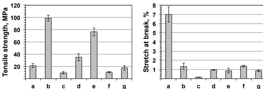
**Fig. 3.** Mechanical properties of bio-based films: (a) BC film (obtained by the solvent exchange method from biosynthesized cellulose), (b) OX-BC film, (c) OX-KP film, (d) CH film, (e) CH-OX-BC film, (f) CH-OX-KP film, and (g) CH-OX-BB film. Data represent the mean  $\pm$  SD of 8 samples.
