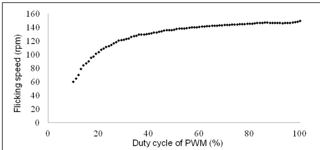
Fig. 2. The effect of duty cycle of PWM to flicking speed.
