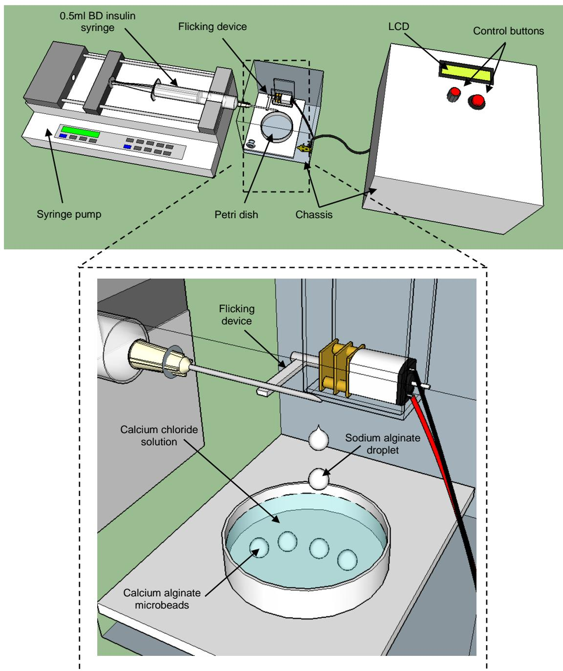
**Fig. 1.** The flicking system for generation of calcium alginate microbeads
