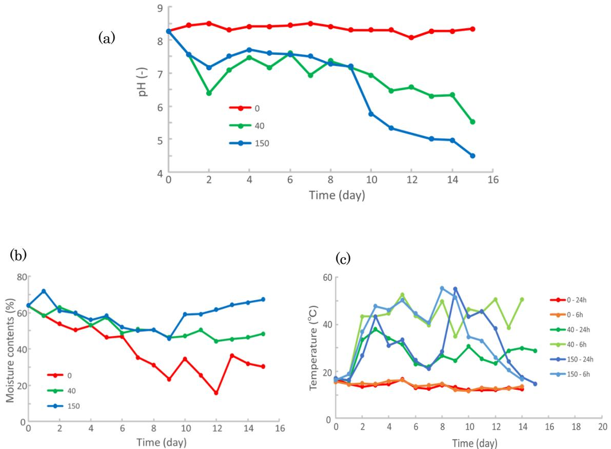
**Fig. 5.** Time course of garbage treatment system (a) pH, (b) Moisture contents, (c) temperature
