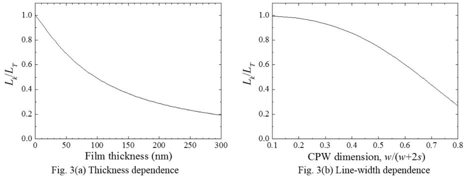
**Fig. 3.** Kinetic inductance in superconducting single-crystal-NbTiN CPW. (a) Film-thickness dependence, (b) CPW-dimension dependence.
