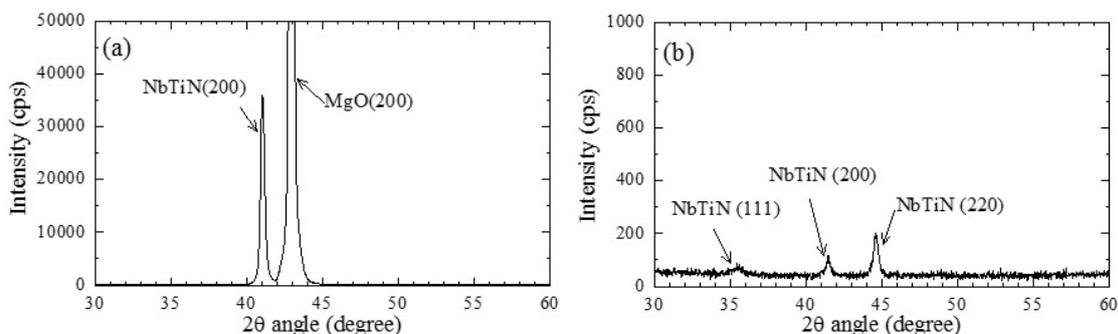
**Fig. 1.** X-ray diffraction patterns of 40-nm-thick NbTiN thin films fabricated on (a) MgO and (b) fused quartz substrates.
