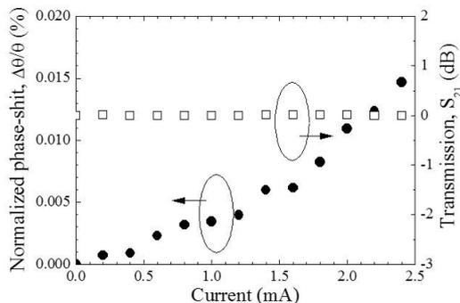
Fig. 6(a) Transmission characteristic
