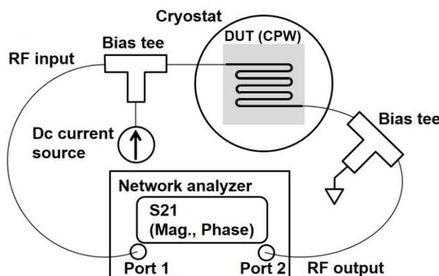
Fig. 5. Measurement setup for the evaluation of nonlinear kinetic inductance.
