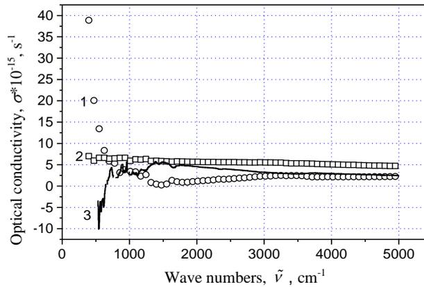
**Fig. 3.** The spectrum of optical conductivity of the surface of polycrystalline Mo before irradiation (curve 1), after irradiation by Ti<sup>+</sup> and C<sup>+</sup> ion-plasma mixed beam (curve 2), and the difference of previous graphs (curve 3) in the IR.
