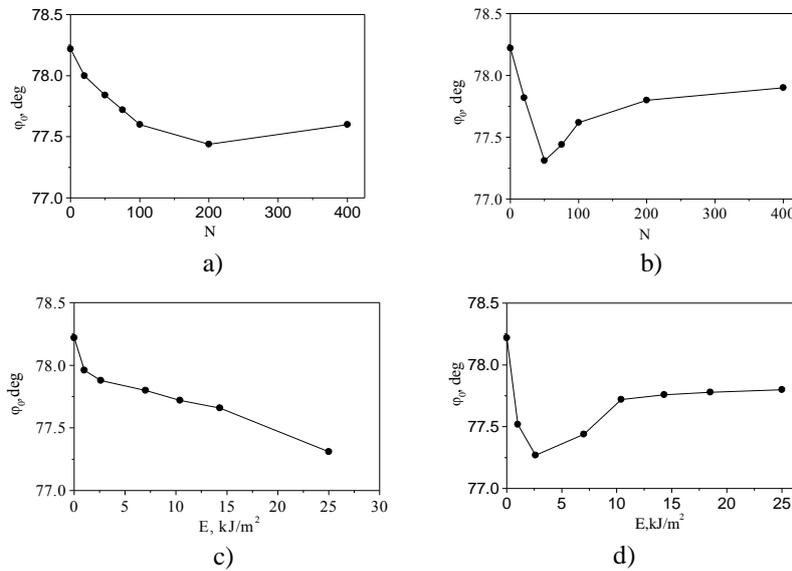
**Fig. 1.** The principal angle of incidence  $\phi_0$  of the Fe-Cr-B ribbons as a function of the number  $N$  of laser pulses ( $E = 7$  (a) and  $25 \text{ kJ/m}^2$  (b)) and laser pulse energy  $E$  ( $N = 50$  (c) and  $200$  (d)).
