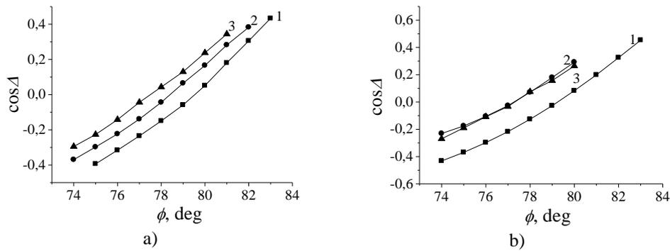
**Fig. 2.** The curves  $\cos\Delta(\varphi)$  of the hypoeutectic (a) and eutectic (b) Al-Si alloy samples as untreated (1), laser treated with J below (2) and above (3) the melting threshold.
