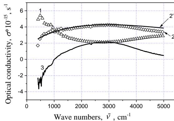
**Fig. 4.** The spectrum of optical conductivity of the surface of polycrystalline Ti before irradiation (curve 1), after irradiation by Ti<sup>+</sup> and C<sup>+</sup> ion-plasma mixed beam (curve 2), the difference of previous graphs (curve 3) in the IR. Curve 2' is a result of the calculation of the optical conductivity in an approximation of Kaveh-Mott relationship (2).
