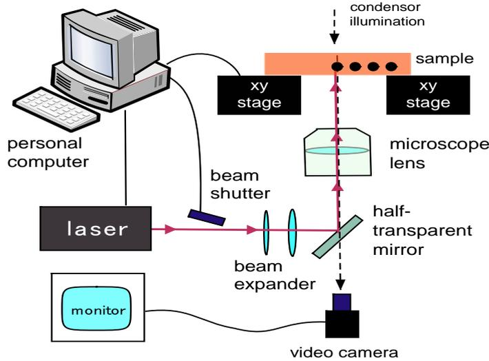
**Fig. 1.** Experimental system for localization encoding using laser-induced damage.
