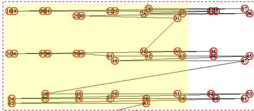
**Fig. 3.** Laser control sequence obtained by direct scan-line conversion of the raster CLUSPI code enclosed in the dashed rectangle in Fig.2(b) with interleaved cluster components.
