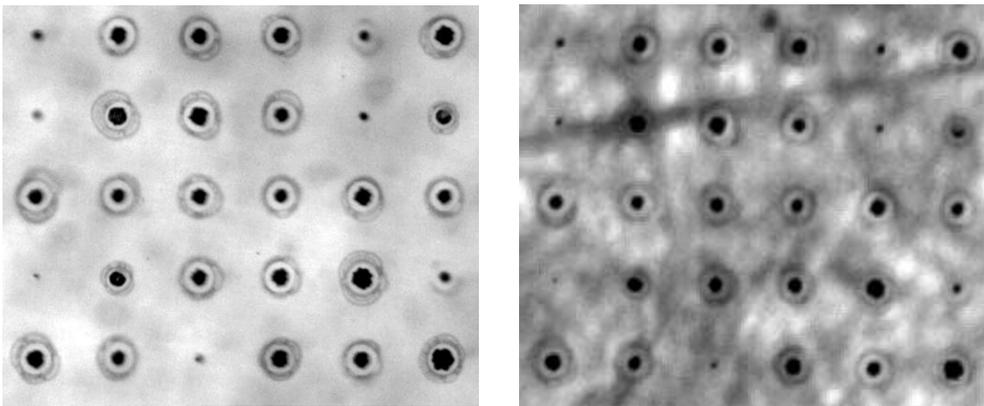
Fig. 7. Optical microscopy images of the dot pattern before the lamination (left) and after it (right).
