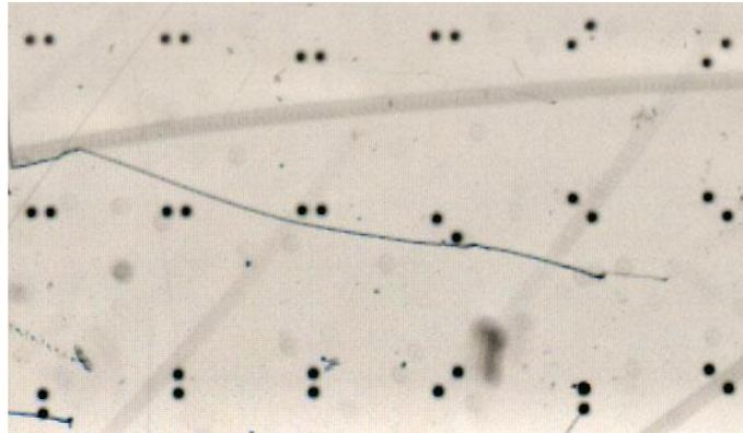
**Fig. 5.** Partial view of a laser-encoded sample after applying the sequences from Table I. The CLUSPI encoded area visible on this sample is highlighted in Fig.2(b) and in Figs 3 and 4.
