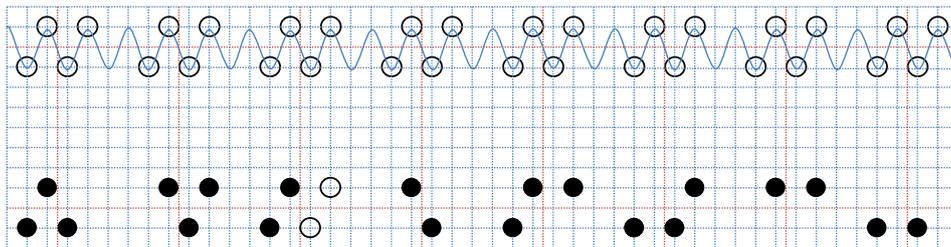
**Fig. 6.** Sample cluster code pattern specifically designed for efficient laser marking. The laser beam follows a sine path (top row) and shots a fired at selected peaks of the sine wave (top hollow circles). Valid clusters are shown in the bottom row.
