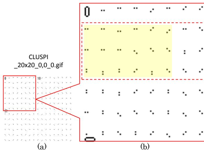
**Fig. 2.** A 20x20 CLUSPI-encoded surface patch (a) and an enlargement of its top left corner (b).
