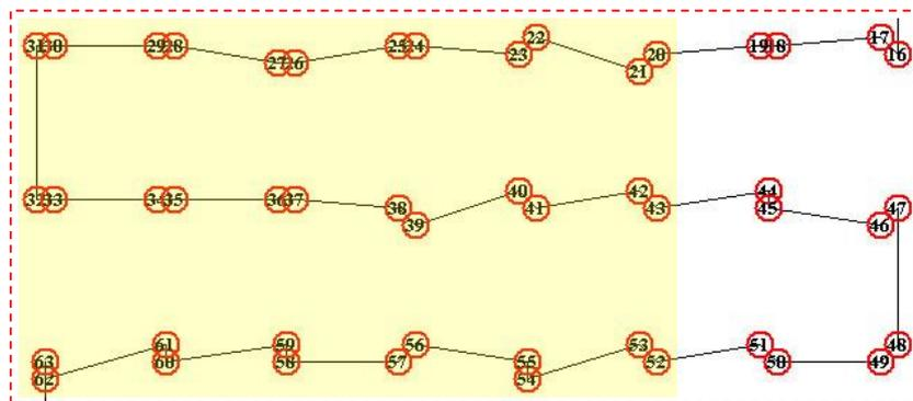
**Fig. 4.** A laser control sequence for the raster CLUSPI code enclosed in the dashed rectangle in Fig.2(b) with consecutive cluster encoding and no interleaved cluster components.
