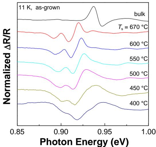
Figure 4 PR spectra of as-grown films.
