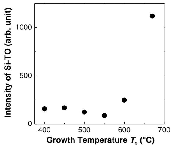
Figure 2 Intensity of Si-TO line as a function of growth temperature.
