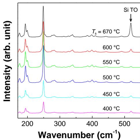
Figure 1 Raman spectra grown at different growth temperatures.
