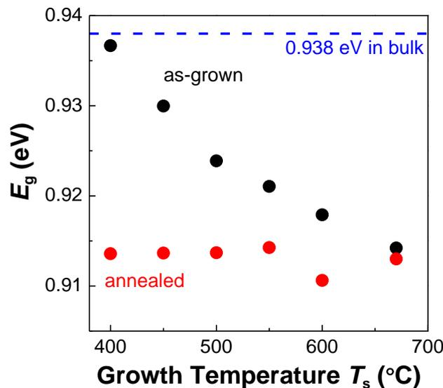
Figure 6 Direct transition energy ( $E_g$ ) as a function of growth temperature.
