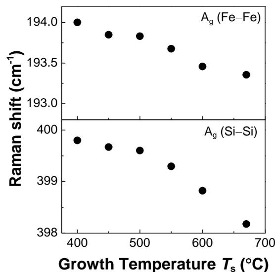
Figure 3 Raman peak positions of  $A_g$ -mode as a function of growth temperature.
