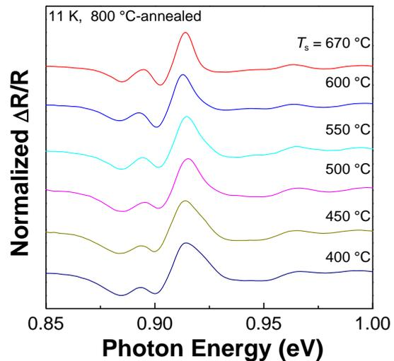
Figure 5 PR spectra of films annealed at  $800\text{ }^\circ\text{C}$ .
