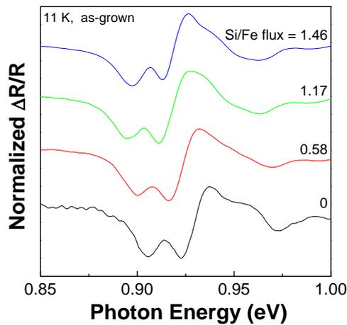
Figure 7 PR spectra of as-grown films.
