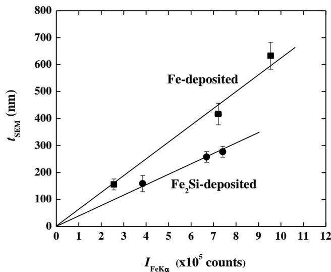
**Fig. 3.** Plots of the film thickness evaluated by cross sectional SEM ( $t_{\text{SEM}}$ ) versus the integrated intensity of Fe  $K\alpha$  lines ( $I_{\text{Fe}K\alpha}$ ) evaluated by SEM-EDS. Solid squares are for Fe-deposited, and solid circles are for  $\text{Fe}_2\text{Si}$ -deposited.
