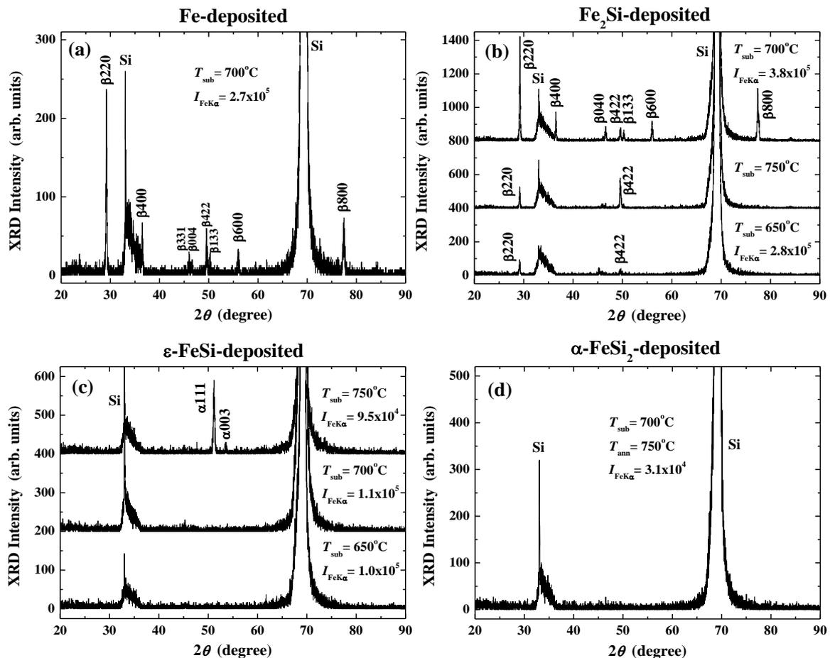
**Fig. 1.** XRD profiles of thin films fabricated in various conditions: (a) Fe-deposited, (b)  $\text{Fe}_2\text{Si}$ -deposited, (c)  $\epsilon\text{-FeSi}$ -deposited, and (d)  $\alpha\text{-FeSi}_2$ -deposited.  $I_{\text{FeK}\alpha}$  represents the integral intensities of Fe K $\alpha$  line from  $1.28 \times 0.96$  mm<sup>2</sup> area of each film by SEM-EDS.
