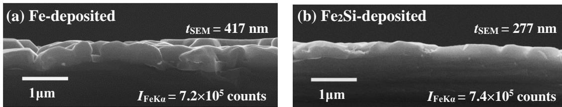
**Fig. 2.** Cross-sectional SEM images of  $\beta\text{-FeSi}_2$  thin films, (a) Fe-deposited, (b)  $\text{Fe}_2\text{Si}$ -deposited.  $t_{\text{SEM}}$  are average thickness of  $\beta\text{-FeSi}_2$  thin films evaluated from the cross-sectional SEM images, and  $I_{\text{Fe}K\alpha}$  represents the EDS peak integral intensities of Fe  $K\alpha$  line from  $1.28 \times 0.96$  mm<sup>2</sup> area of each films.
