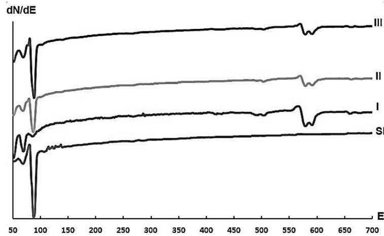
Fig. 1. AES spectra for the samples deposited at 300 K and annealed at 800 °C
