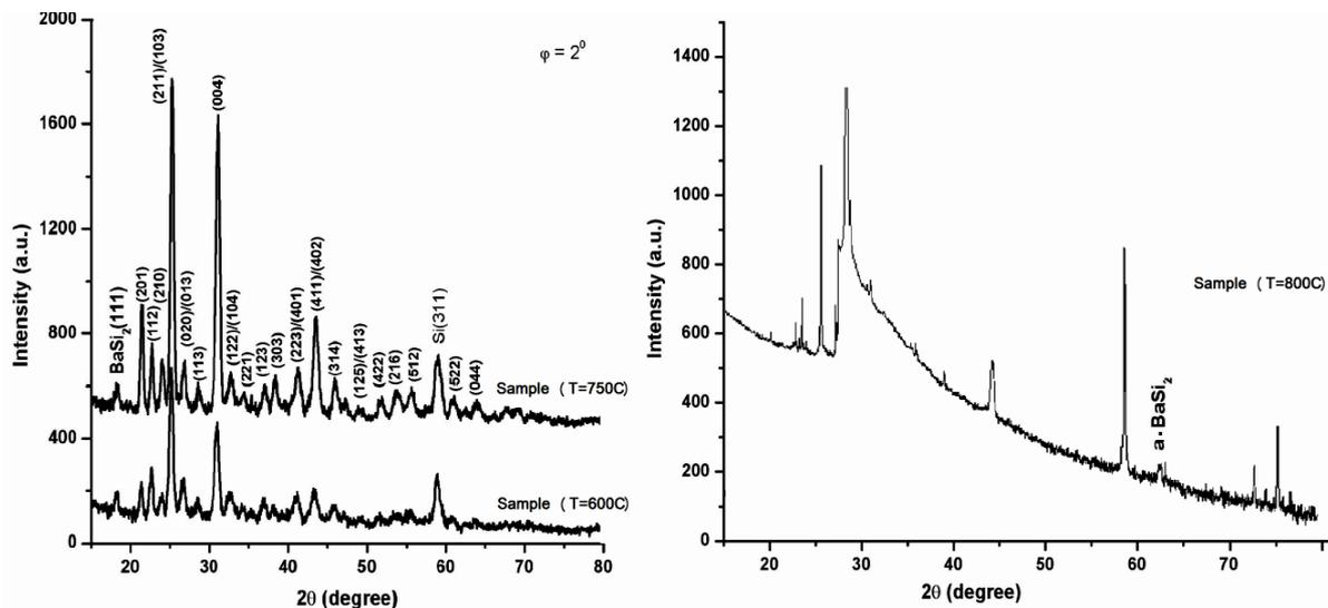
Fig. 2. GIXRD spectra for the samples deposited at 300 K and annealed at 600, 750 and 800 °C and measured at incidence angle  $\phi = 2^\circ$ .
