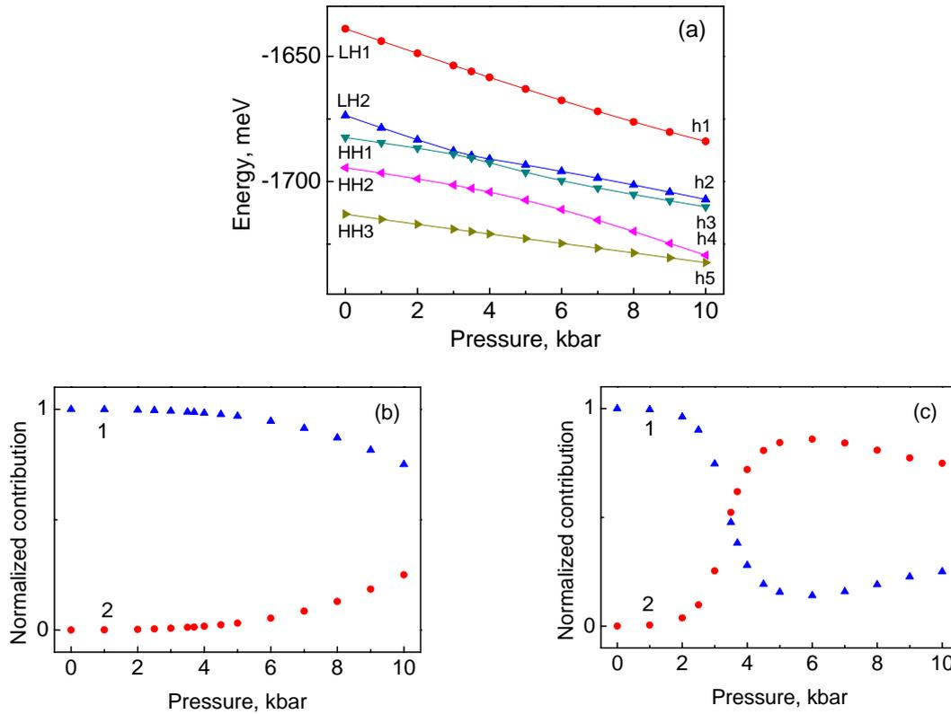
**Fig. 2.** Calculated energy shifts of five hole levels at the zone center under uniaxial compression (a) and pressure dependence of normalized contribution of basis functions with different angular momentum projection  $|m_j| = 1/2$  (1) and  $|m_j| = 3/2$  (2) into wave functions of h1(b) and h2 (c) hole levels for the GaAs<sub>0.84</sub>P<sub>0.16</sub> QW of 14 nm width ( $P \parallel [110]$ ,  $T = 77$  K) [5].
