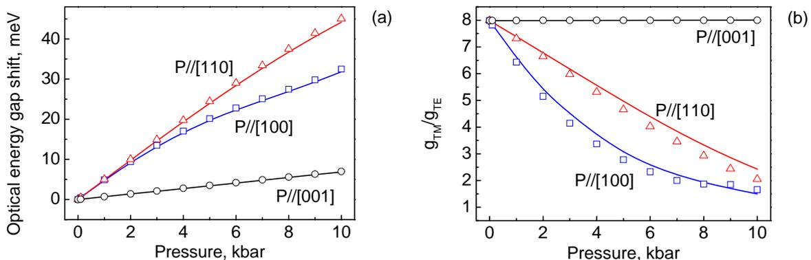
**Fig. 1.** Pressure dependence of the optical energy gap (a) and  $g_{\text{TM}}/g_{\text{TE}}$  ratio (b) for the  $\text{GaAs}_{0.84}\text{P}_{0.16}$  QW of 14 nm width under uniaxial compression along different directions at  $T = 77$  K (lines) and  $T = 300$  K (symbols).
