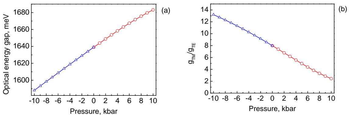
**Fig. 3.** Pressure dependence of the optical energy gap (a) and  $g_{TM}/g_{TE}$  ratio (b) for the GaAs<sub>0.84</sub>P<sub>0.16</sub> QW of 14 nm width under uniaxial compression (circles) and tension (triangles) along [110] direction at  $T = 77$  K.
