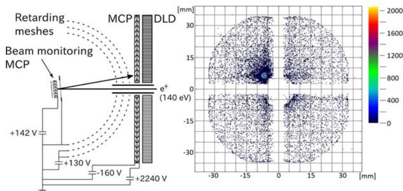
**Fig. 3** (Left) A beam monitoring MCP assembly with a fluorescent screen and a grounded mesh in front of the MCP front. This assembly was slightly tilted against the incident beam trajectory and also used as an electrostatic mirror by applying an electrostatic potential to the MCP front at a slightly higher voltage than the beam energy. The potential values correspond to a beam energy of 140 eV. (Right) The deflected beam observed by the MCP-DLD.
