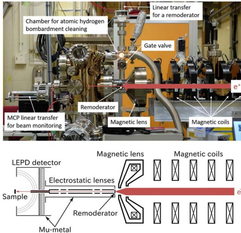
**Fig. 2** Photo of the LEPD station (above) and a diagram of the brightness enhancement system, electrostatic lenses for transporting the remoderated beam, and the LEPD detector (bottom). These electrostatic lenses and the detector are covered by a permalloy cylinder. The thin nozzle on the left hand side of the figure goes through the center holes of the MCP and the DLD.
