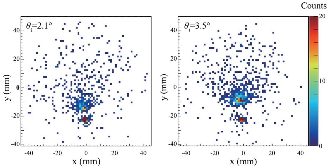
**Fig. 3** Spatial profiles of the Ps atoms scattered at the incident angle of  $2.1^\circ$  (left) and  $3.5^\circ$  (right).
