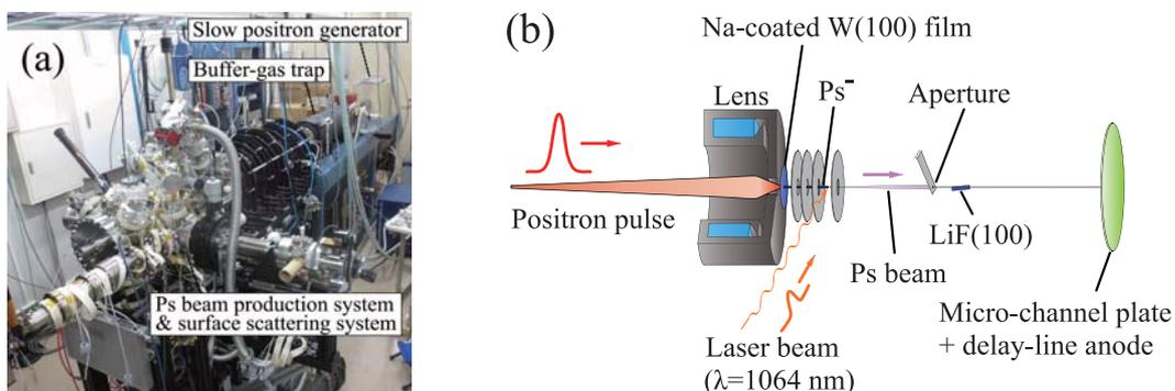
**Fig. 1** (a) Photograph of the Ps beam apparatus at the Tokyo University of Science, (b) schematic diagram of the Ps beam production system and the setup for the surface scattering experiment.
