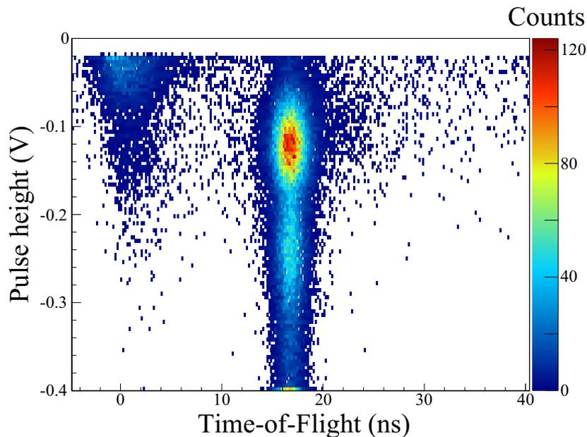
**Fig. 2** 2-dimensional Time-of-Flight and pulse-height distribution of the detected signals, accumulated over 1800 s.
